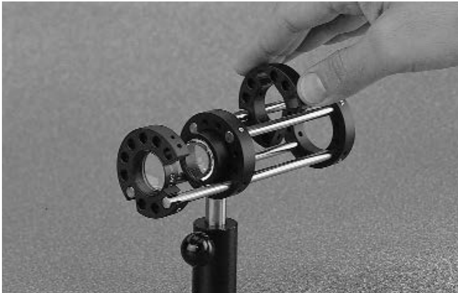
The two-rod insertion plate (50-102) and four-rod insertion plate (50-148) have open support rod mounting holes that permit their insertion into assemblies without disturbing the system. Also shown is post mount 50-126.
