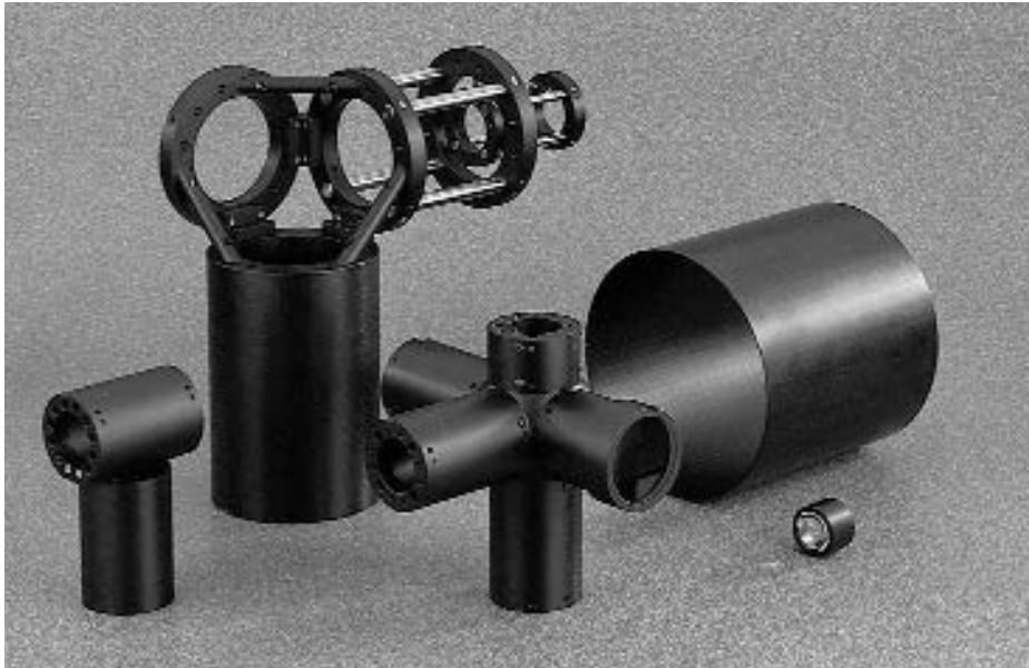
Support tubes allow long optical path-lengths and utilization of larger optics. Shown above is a 50 mm MICROPTIC lens mount attached to a 5-way node. A 3-way node is shown on the left. Oblique rods (rear) maintain rigidity at the node.
