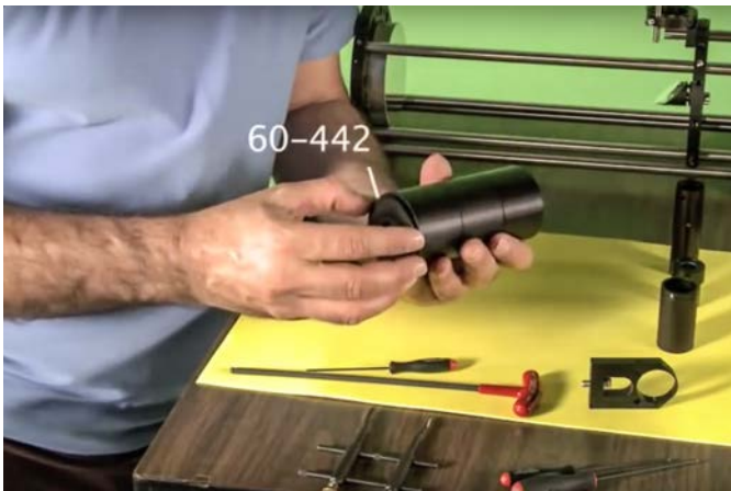
End plate 60-422 is added to one end
