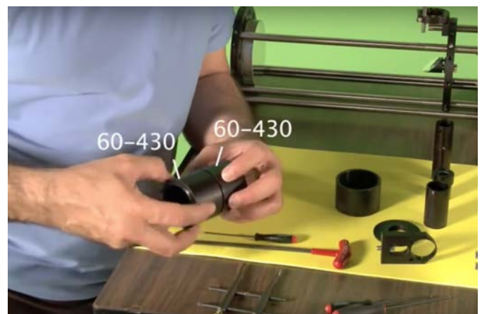
To secure the tubes, the connecting ring is held by nail
