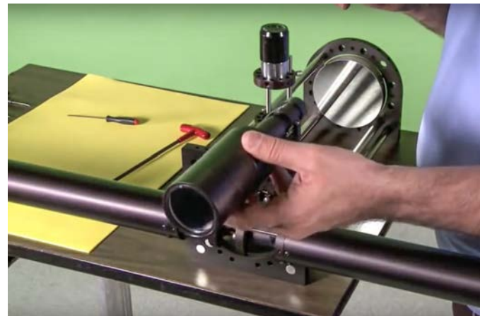
The finder scope is inserted into the mounting column
