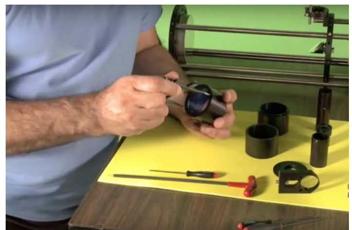
A spanner wrench is needed to secure the rings
