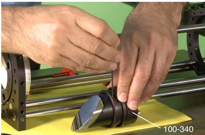
Stepping up Minioptic 100 accessories, i.e., 100-340 to fit inside Macroptic 150 mounts via Macroptic 150 centering ring 150-160.
