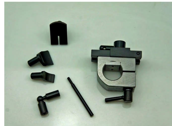
Traditional watchmaking lathe bed (still manufactured by French, Bergeon) resembles the new A-Line product by Newport. Newport's innovation was to use a set screw to both align, and secure the quick-release mounts.
