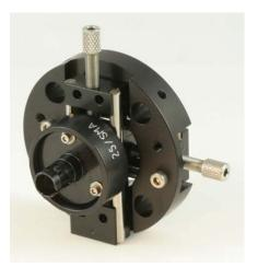
20-508 SMA Connector with X-Y
