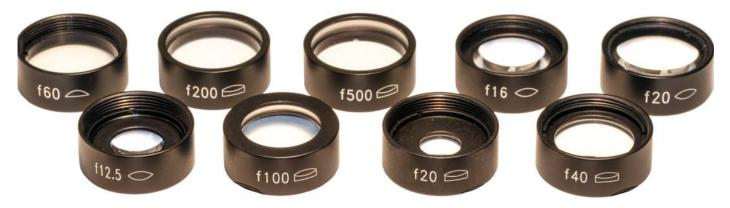
While inside optics cells, optical elements are easily identifiable, they are unscratchable, they are easy to use, they are easy to store, and the optics will stay clean because they are not touched by hands. They are also centered inside the mounts with reasonable seating tolerances + / - 0.07 mm. Mounting tolerance of 25 mm lens cells placed inside Optoform mounts is better than + / - 0.05 mm. The centration of Microptic 50 mounts along the rods is better than + / - 0.02.
