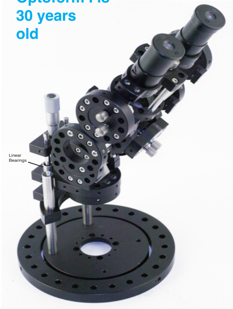
Optoform I introduced linear bearings: It consists of a stationary plate, and a translation plate pushed by micrometer.
